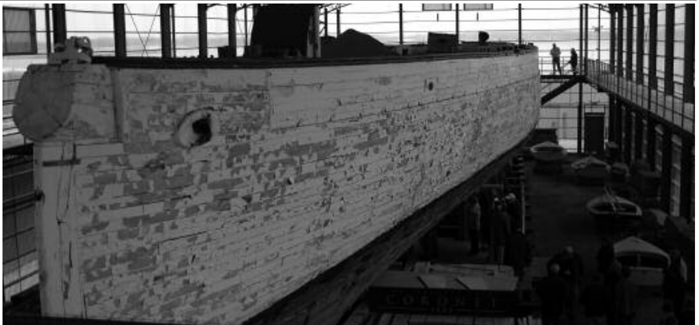
The restorers figure that they will be able to keep 80% of the exterior planks
